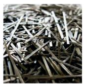
The basalt stones are heated up to 1450 degrees Celcius. The liquid mass is then pressed through nozzles to give long fibers. After the fibers are cooled down we can begin to create the furniture. Bio-resin bind the fibers together.
